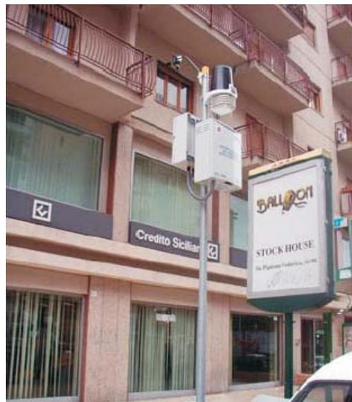
The ETL 2000 provides quality data utilising a central station software @COM3000 remotely retrieving data via landline modem or GSM, either from a single ETL or a network of units.
